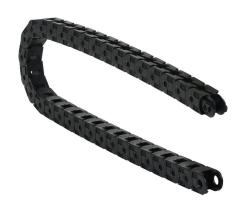
Murrplastik MP10 cable drag chain, 0.39in inside height, 0.24in inside width, 1.1in bend radius, outside opening, 0.59in pitch, 1.6ft/0.5m length, black. Requires CDC-KAZ-04X02 bracket for mounting.
