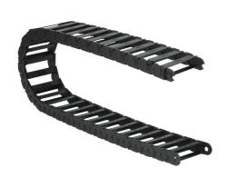
Murrplastik MP18 cable drag chain, 0.71in inside height, 2.76in inside width, 3.07in bend radius, outside opening, 1.3in pitch, 3.2ft/1m length, black. Requires CDC-KAZ-0.7X2.8 bracket for mounting.
