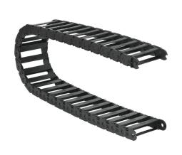
Murrplastik MP18 cable drag chain, 0.71in inside height, 2.76in inside width, 3.07in bend radius, inside opening, 1.3in pitch, 3.2ft/1m length, black. Requires CDC-KAZ-0.7X2.8 bracket for mounting.
