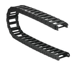
Murrplastik MP18 cable drag chain, 0.71in inside height, 1.97in inside width, 3.07in bend radius, outside opening, 1.3in pitch, 3.2ft/1m length, black. Requires CDC-KAZ-0.7X2.0 bracket for mounting.
