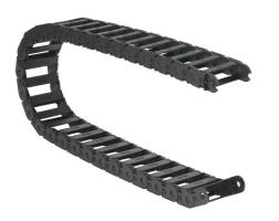
Murrplastik MP18 cable drag chain, 0.71in inside height, 1.97in inside width, 3.07in bend radius, inside opening, 1.3in pitch, 3.2ft/1m length, black. Requires CDC-KAZ-0.7X2.0 bracket for mounting.
