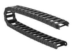
Murrplastik MP18 cable drag chain, 0.71in inside height, 1.97in inside width, 1.89in bend radius, outside opening, 1.3in pitch, 3.2ft/1m length, black. Requires CDC-KAZ-0.7X2.0 bracket for mounting.
