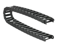
Murrplastik MP18 cable drag chain, 0.71in inside height, 1.97in inside width, 1.89in bend radius, inside opening, 1.3in pitch, 3.2ft/1m length, black. Requires CDC-KAZ-0.7X2.0 bracket for mounting.
