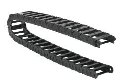
Murrplastik MP18 cable drag chain, 0.71in inside height, 1.97in inside width, 1.5in bend radius, outside opening, 1.3in pitch, 3.2ft/1m length, black. Requires CDC-KAZ-0.7X2.0 bracket for mounting.
