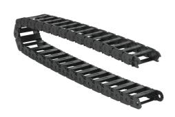
Murrplastik MP18 cable drag chain, 0.71in inside height, 1.97in inside width, 1.5in bend radius, inside opening, 1.3in pitch, 3.2ft/1m length, black. Requires CDC-KAZ-0.7X2.0 bracket for mounting.
