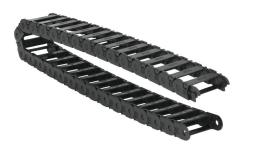
Murrplastik MP18 cable drag chain, 0.71in inside height, 1.97in inside width, 1.1in bend radius, outside opening, 1.3in pitch, 3.2ft/1m length, black. Requires CDC-KAZ-0.7X2.0 bracket for mounting.
