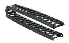
Murrplastik MP18 cable drag chain, 0.71in inside height, 1.97in inside width, 1.1in bend radius, inside opening, 1.3in pitch, 3.2ft/1m length, black. Requires CDC-KAZ-0.7X2.0 bracket for mounting.
