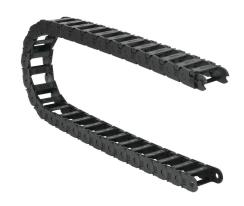
Murrplastik MP18 cable drag chain, 0.71in inside height, 1.46in inside width, 3.07in bend radius, outside opening, 1.3in pitch, 3.2ft/1m length, black. Requires CDC-KAZ-0.7X1.5 bracket for mounting.
