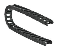
Murrplastik MP18 cable drag chain, 0.71in inside height, 1.46in inside width, 3.07in bend radius, inside opening, 1.3in pitch, 3.2ft/1m length, black. Requires CDC-KAZ-0.7X1.5 bracket for mounting.
