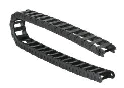
Murrplastik MP18 cable drag chain, 0.71in inside height, 1.46in inside width, 1.89in bend radius, outside opening, 1.3in pitch, 3.2ft/1m length, black. Requires CDC-KAZ-0.7X1.5 bracket for mounting.
