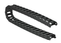
Murrplastik MP18 cable drag chain, 0.71in inside height, 1.46in inside width, 1.89in bend radius, inside opening, 1.3in pitch, 3.2ft/1m length, black. Requires CDC-KAZ-0.7X1.5 bracket for mounting.
