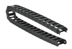
Murrplastik MP18 cable drag chain, 0.71in inside height, 1.46in inside width, 1.5in bend radius, outside opening, 1.3in pitch, 3.2ft/1m length, black. Requires CDC-KAZ-0.7X1.5 bracket for mounting.
