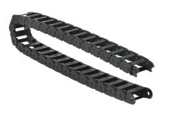
Murrplastik MP18 cable drag chain, 0.71in inside height, 1.46in inside width, 1.5in bend radius, inside opening, 1.3in pitch, 3.2ft/1m length, black. Requires CDC-KAZ-0.7X1.5 bracket for mounting.
