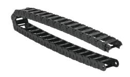
Murrplastik MP18 cable drag chain, 0.71in inside height, 1.46in inside width, 1.1in bend radius, outside opening, 1.3in pitch, 3.2ft/1m length, black. Requires CDC-KAZ-0.7X1.5 bracket for mounting.
