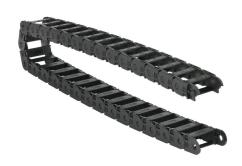
Murrplastik MP18 cable drag chain, 0.71in inside height, 1.46in inside width, 1.1in bend radius, inside opening, 1.3in pitch, 3.2ft/1m length, black. Requires CDC-KAZ-0.7X1.5 bracket for mounting.
