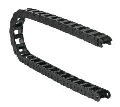
Murrplastik MP18 cable drag chain, 0.71in inside height, 0.98in inside width, 3.07in bend radius, outside opening, 1.3in pitch, 3.2ft/1m length, black. Requires CDC-KAZ-0.7X1.0 bracket for mounting.
