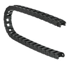
Murrplastik MP18 cable drag chain, 0.71in inside height, 0.98in inside width, 3.07in bend radius, inside opening, 1.3in pitch, 3.2ft/1m length, black. Requires CDC-KAZ-0.7X1.0 bracket for mounting.
