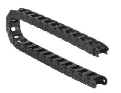
Murrplastik MP18 cable drag chain, 0.71in inside height, 0.98in inside width, 1.89in bend radius, inside opening, 1.3in pitch, 3.2ft/1m length, black. Requires CDC-KAZ-0.7X1.0 bracket for mounting.
