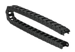
Murrplastik MP18 cable drag chain, 0.71in inside height, 0.98in inside width, 1.5in bend radius, outside opening, 1.3in pitch, 3.2ft/1m length, black. Requires CDC-KAZ-0.7X1.0 bracket for mounting.
