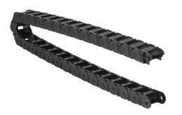
Murrplastik MP18 cable drag chain, 0.71in inside height, 0.98in inside width, 1.1in bend radius, outside opening, 1.3in pitch, 3.2ft/1m length, black. Requires CDC-KAZ-0.7X1.0 bracket for mounting.
