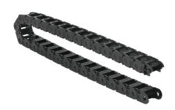
Murrplastik MP18 cable drag chain, 0.71in inside height, 0.98in inside width, 1.1in bend radius, inside opening, 1.3in pitch, 3.2ft/1m length, black. Requires CDC-KAZ-0.7X1.0 bracket for mounting.
