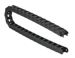
Murrplastik MP18 cable drag chain, 0.71in inside height, 0.71in inside width, 1.89in bend radius, outside opening, 1.3in pitch, 3.2ft/1m length, black. Requires CDC-KAZ-0.7X0.7 bracket for mounting.
