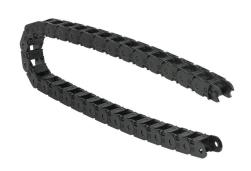
Murrplastik MP18 cable drag chain, 0.71in inside height, 0.71in inside width, 1.89in bend radius, inside opening, 1.3in pitch, 3.2ft/1m length, black. Requires CDC-KAZ-0.7X0.7 bracket for mounting.
