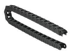
Murrplastik MP18 cable drag chain, 0.71in inside height, 0.71in inside width, 1.5in bend radius, outside opening, 1.3in pitch, 3.2ft/1m length, black. Requires CDC-KAZ-0.7X0.7 bracket for mounting.
