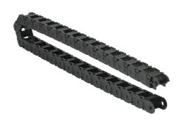
Murrplastik MP18 cable drag chain, 0.71in inside height, 0.71in inside width, 1.1in bend radius, outside opening, 1.3in pitch, 3.2ft/1m length, black. Requires CDC-KAZ-0.7X0.7 bracket for mounting.
