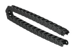
Murrplastik MP18 cable drag chain, 0.71in inside height, 0.71in inside width, 1.1in bend radius, inside opening, 1.3in pitch, 3.2ft/1m length, black. Requires CDC-KAZ-0.7X0.7 bracket for mounting.
