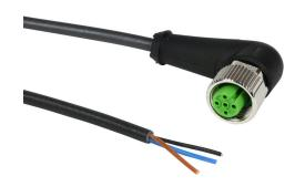
AutomationDirect connection cable, M12 right-angle female to pigtail, 3-pole, PUR jacket, black, 16.4ft/5m cable length, IP67.
