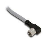
AutomationDirect connection cable, M8 right-angle female to pigtail, 4-pole, PVC jacket, black, 32.8ft/10m cable length, IP67.
