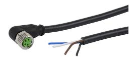
AutomationDirect connection cable, M8 right-angle female to pigtail, 4-pole, PVC jacket, black, 16.4ft/5m cable length, IP67.
