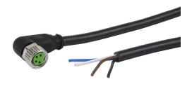
AutomationDirect connection cable, M8 right-angle female to pigtail, 4-pole, PVC jacket, black, 16.4ft/5m cable length, IP67.
