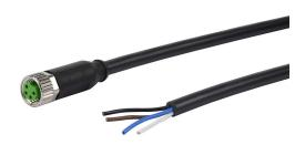
AutomationDirect connection cable, M8 axial female to pigtail, 4-pole, PVC jacket, black, 6.5ft/2m cable length, IP67.
