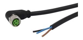
AutomationDirect connection cable, M8 right-angle female to pigtail, 3-pole, PUR jacket, black, 16.4ft/5m cable length, IP67.
