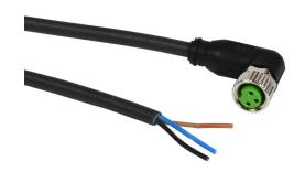
AutomationDirect connection cable, M8 right-angle female to pigtail, 3-pole, PUR jacket, black, 16.4ft/5m cable length, IP67.
