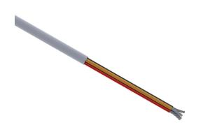
Quabbin control cable, unshielded, 4 conductors, 20 AWG, 7-stranded, tinned copper, PVC conductor insulation material, PVC jacket, gray, cut to length.
