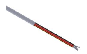
Quabbin control cable, unshielded, 3 conductors, 20 AWG, 7-stranded, tinned copper, PVC conductor insulation material, PVC jacket, gray, cut to length.
