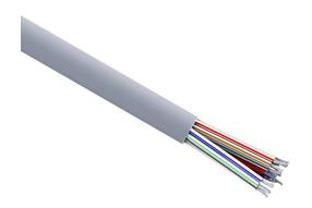
Quabbin control cable, unshielded, 25 conductors, 20 AWG, 7-stranded, tinned copper, PVC conductor insulation material, PVC jacket, gray, cut to length.
