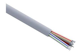
Quabbin control cable, unshielded, 25 conductors, 20 AWG, 7-stranded, tinned copper, PVC conductor insulation material, PVC jacket, gray, cut to length.
