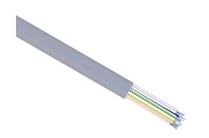
Quabbin control cable, unshielded, 19 conductors, 20 AWG, 7-stranded, tinned copper, PVC conductor insulation material, PVC jacket, gray, cut to length.
