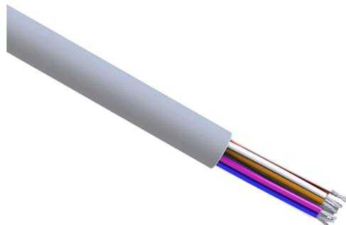
Quabbin control cable, unshielded, 15 conductors, 20 AWG, 7-stranded, tinned copper, PVC conductor insulation material, PVC jacket, gray, cut to length.
