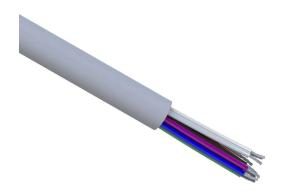
Quabbin flexible control cable, unshielded, 12 conductors, 20 AWG, 7-stranded, tinned copper, PVC conductor insulation material, PVC jacket, gray, cut to length.
