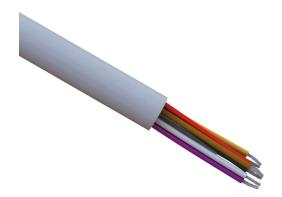
Quabbin control cable, unshielded, 9 conductors, 18 AWG, 16-stranded, tinned copper, PVC conductor insulation material, PVC jacket, gray, cut to length.
