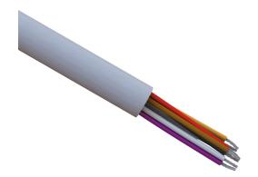
Quabbin control cable, unshielded, 9 conductors, 18 AWG, 16-stranded, tinned copper, PVC conductor insulation material, PVC jacket, gray, cut to length.
