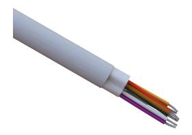
Quabbin control cable, shielded, 9 conductors, 18 AWG, 16-stranded, tinned copper, PVC conductor insulation material, PVC jacket, gray, cut to length.
