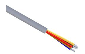
Quabbin control cable, unshielded, 7 conductors, 18 AWG, 16-stranded, tinned copper, PVC conductor insulation material, PVC jacket, gray, cut to length.
