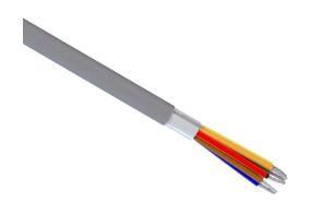
Quabbin control cable, shielded, 7 conductors, 18 AWG, 16-stranded, tinned copper, PVC conductor insulation material, PVC jacket, gray, cut to length.
