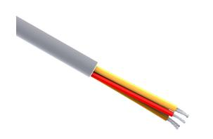
Quabbin control cable, unshielded, 5 conductors, 18 AWG, 16-stranded, tinned copper, PVC conductor insulation material, PVC jacket, gray, cut to length.
