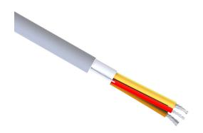
Quabbin control cable, shielded, 5 conductors, 18 AWG, 16-stranded, tinned copper, PVC conductor insulation material, PVC jacket, gray, cut to length.
