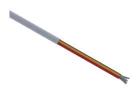
Quabbin control cable, unshielded, 4 conductors, 18 AWG, 16-stranded, tinned copper, PVC conductor insulation material, PVC jacket, gray, cut to length.
