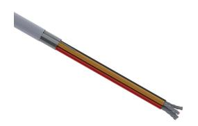
Quabbin control cable, shielded, 4 conductors, 18 AWG, 16-stranded, tinned copper, PVC conductor insulation material, PVC jacket, gray, cut to length.
